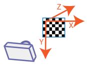
When you reconstruct a 3-D scene from multiple views containing a calibration pattern, the resulting 3-D points are defined in the pattern-based coordinate system. The "Structure From Motion From Two Views" example shows how to reconstruct a 3-D scene from a pair of 2-D images containing a checkerboard pattern.
