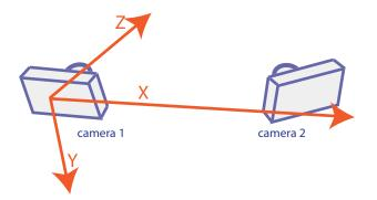
In a stereo system, the origin is located at the optical center of Camera 1.
